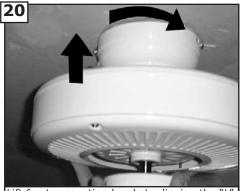
Lift fan to mounting bracket, aligning the "L" shape holes with the scresws on the mounting bracket. Turn the fan clockwise to lock in position. Re-install the screws removed in the previous step and tighten securely.
